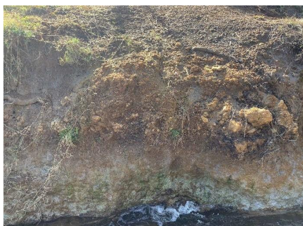
A creek incision reveled a soil profile of residual clay soils and weathered basalt.
